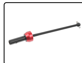
C-00180-360 CVD Drive Shaft - Short - Front - 1 Pc
